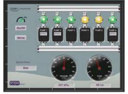
Key information including variable speed status, motor speed, system pressure & flow is clearly displayed on main screen (viewable via the internet).
